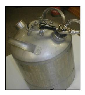
Chemical solution should remain in the draught line for a minimum of 20 minutes.
