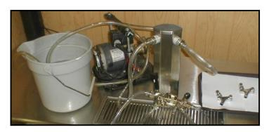
Fill a bucket ("water bucket") with warm water and place the "in" hose into the water.
