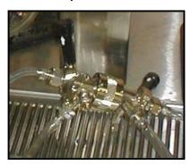
If cleaning four lines, connect a second set of lines with another cleaning coupler, creating a second "loop."
