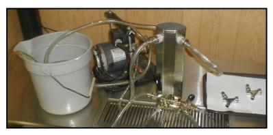
Cleaning flow rate is 2 gallons per minute (2X beer flow rate) Goal is any rate higher than normal flow rate.
