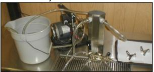
Continue pumping cold water from the water bucket into the chemical bucket (shutting off pump and dumping chemical bucket as needed) until all chemical has been pushed out of the draught lines and there is no solid matter in the rinse water.
